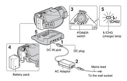
You can charge the "InfoLITHIUM" battery pack (H series) (p. 92) after attaching it to your camcorder.
