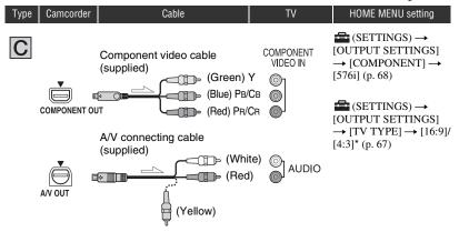
An A/V connecting cable is also needed to output audio signals. Connect the white and red plugs of the A/V connecting cable to the audio input jack of your TV.
