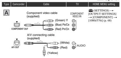
An A/V connecting cable is also needed to output audio signals. Connect the white and red plugs of the A/V connecting cable to the audio input jack of your TV.
